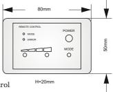
FUNCTIONS of control buttons of the wired remote control POWER — Turning the device ON/OFF.
